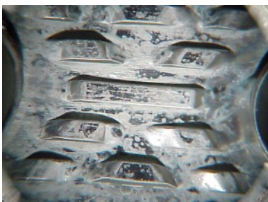
Aluminum fin etched with a foaming action cleaner
